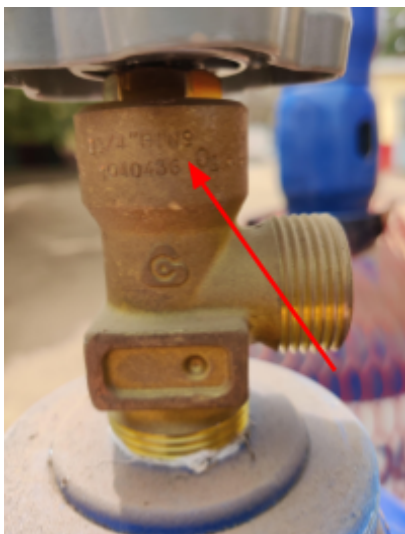
Figure 9 & 10: German valve examples with identifying markers
