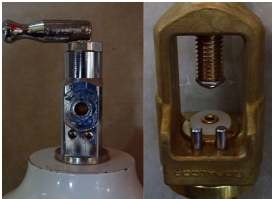
Figure 6: Pin Index Safety System Numbers
