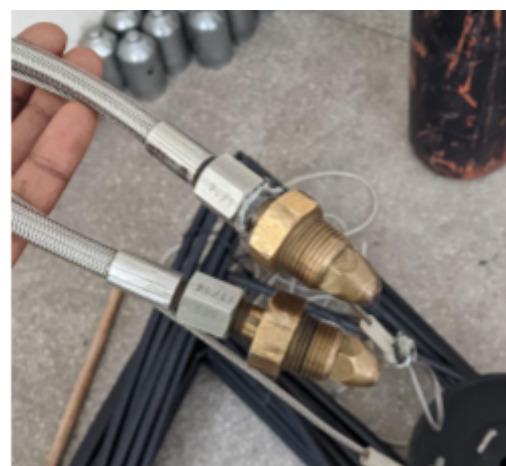
Figure 2: Two British (BS341 #3) cylinder whips from a manifold
