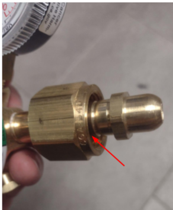
Note the CGA540 markings on the nut
